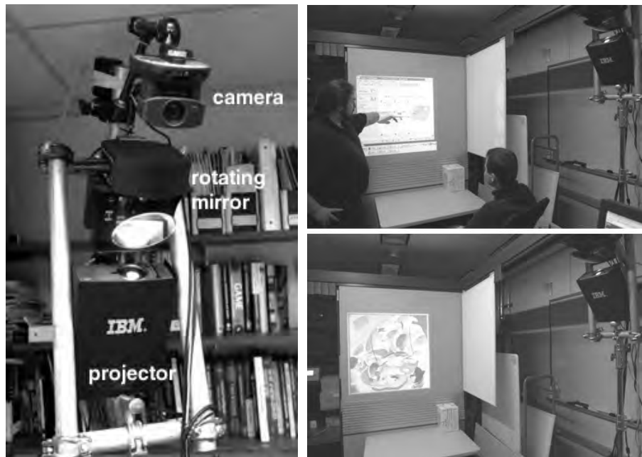
Fig. 2. Current prototype of the Everywhere Displays projector (left) and the projector being used in an office-like environment (right).
