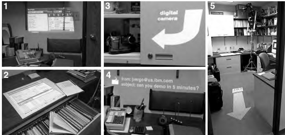
Fig. 9. Augmented reality applications of Everywhere Displays: (1) an electronic phone directory is projected close to the phone; (2) the database corresponding to a file cabinet is accessed directly from the top of the cabinet; (3) a localization system points to the position of an object; (4) a notification of the arrival of an urgent e-mail is silently projected on the wall; (5) an emergency sign projected on the floor directly points to the nearest exit.
