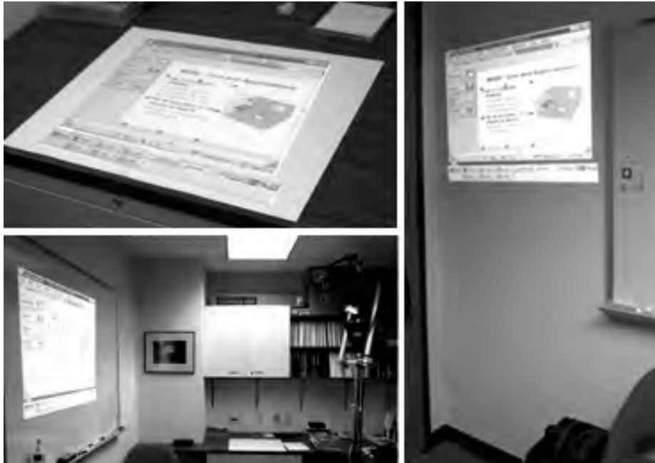
Fig. 8. The ED-projector moving a desktop application to the top of a table, to a whiteboard, and to a wall on the side of the whiteboard.
