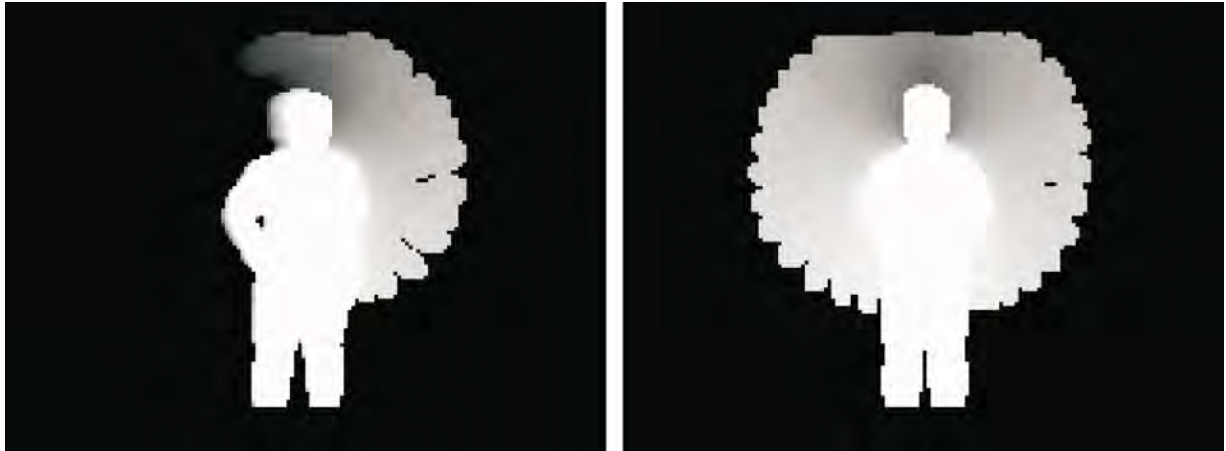
Figure 7 Motion templates used by PAT for recognizing “left-arm stretch” and “deep-breathing stretch”
