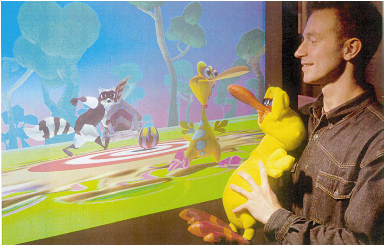
Figure 9 User in front of the screen of Swamped! controlling the computer graphics character by manipulating the plush doll
