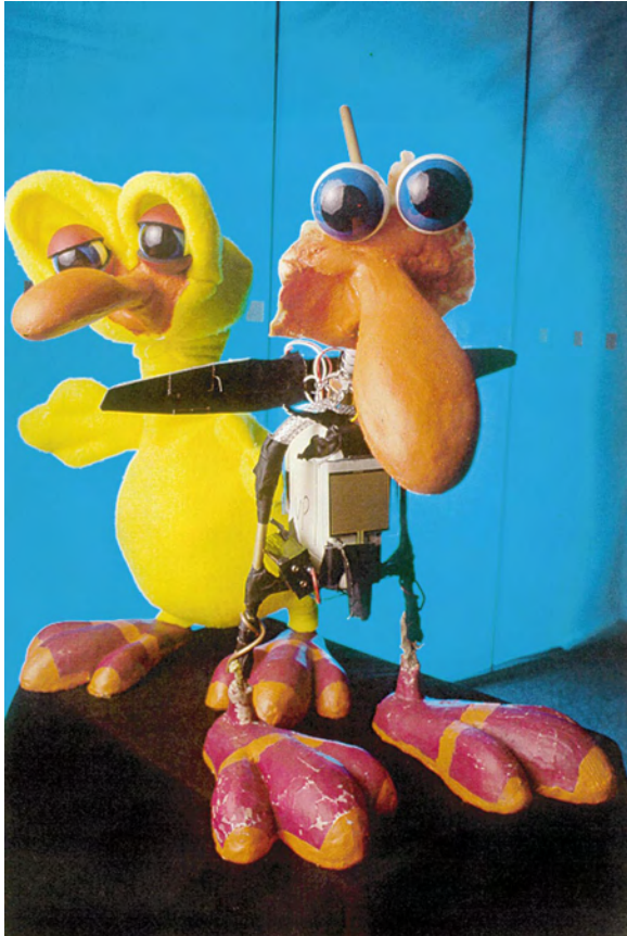
Figure 11 Sensor package installed in the physical doll interface used in Swamped!
