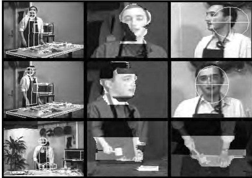
Figure 2: World and view representations: the left column contains the projection of the 3D-model representing the chef in some frames, and the middle and right columns present the view-representations of the head or the hands according to different cameras. In the first and second rows, the cameras were asked to “close-up chef”; in the third row, the calls were “close-up hands”.
