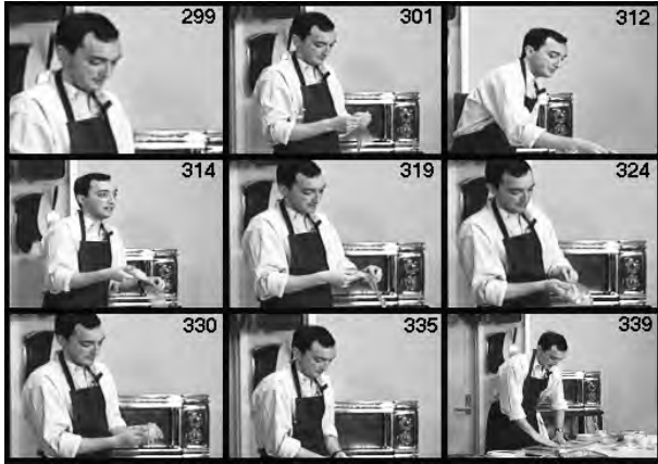
Figure 8: Response of the lateral SmartCam to the call “medium-close-shot chef”; refer to the microwave oven in the background to observe the corrections performed by the camera.
